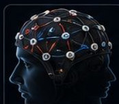
EEG CAP / ELECTRODES Ag/AgCl electrodes capture brain signals.
